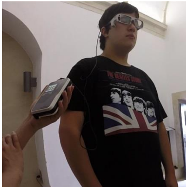
Figure 2 - Calibration of the Tobii Glasses Eyetracker Smart IR.
